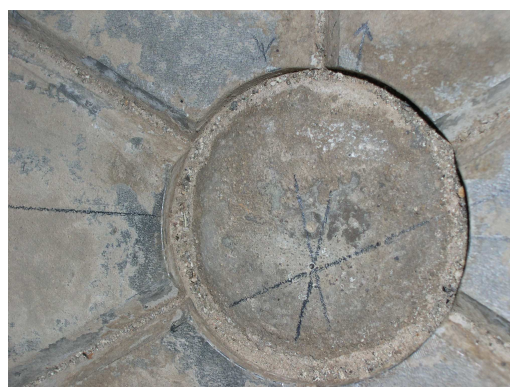
SLR System Reference Point (SRP)
