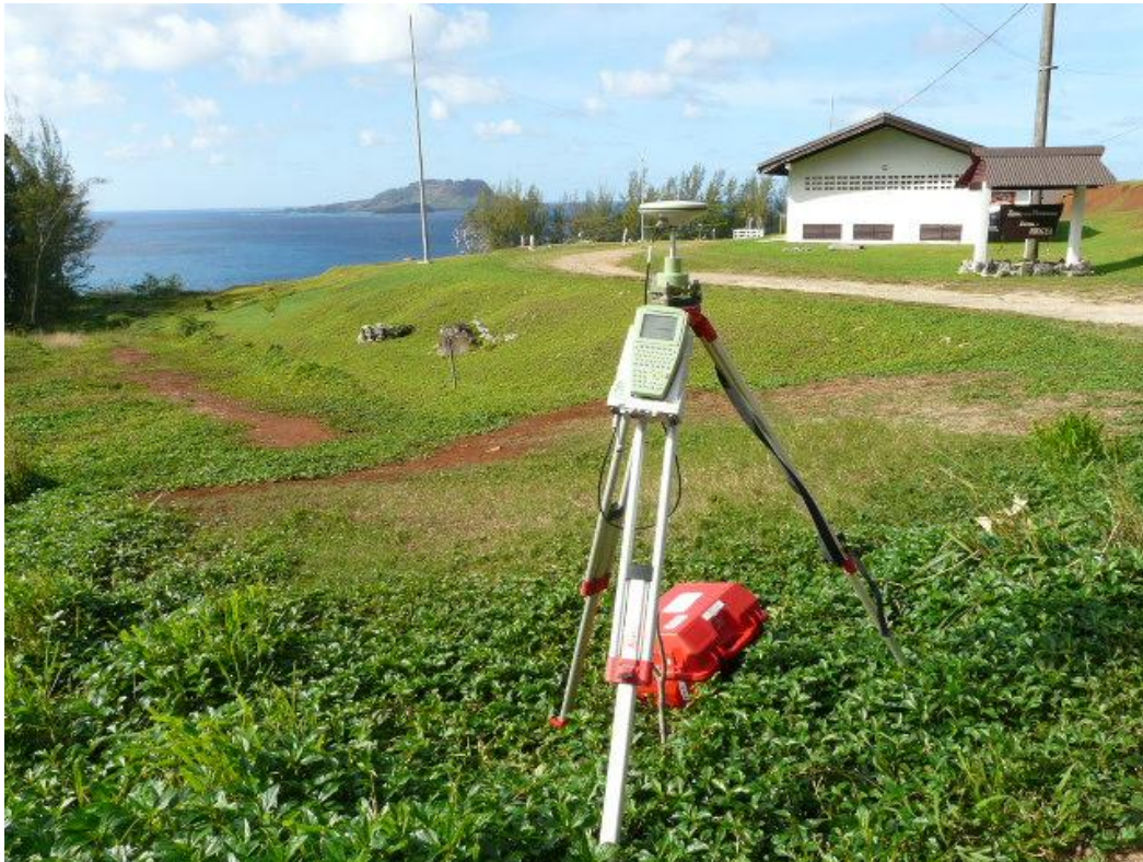
General view of the site with a GNSS station above RefN point in the foreground.
