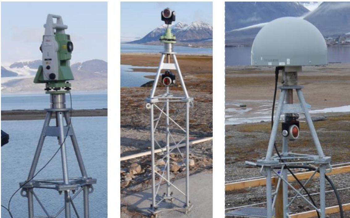
Figure 10 From left: NABG with total station, NABG with prism and NABG_U, NABG GNSS and NABG_U
