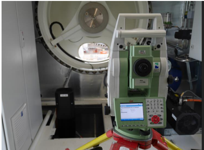
Figure 9 Total station inside azimuth cabin
