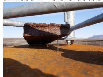
Figure 13 Marker in ground plate, a nail in the hole to make the observations easier
