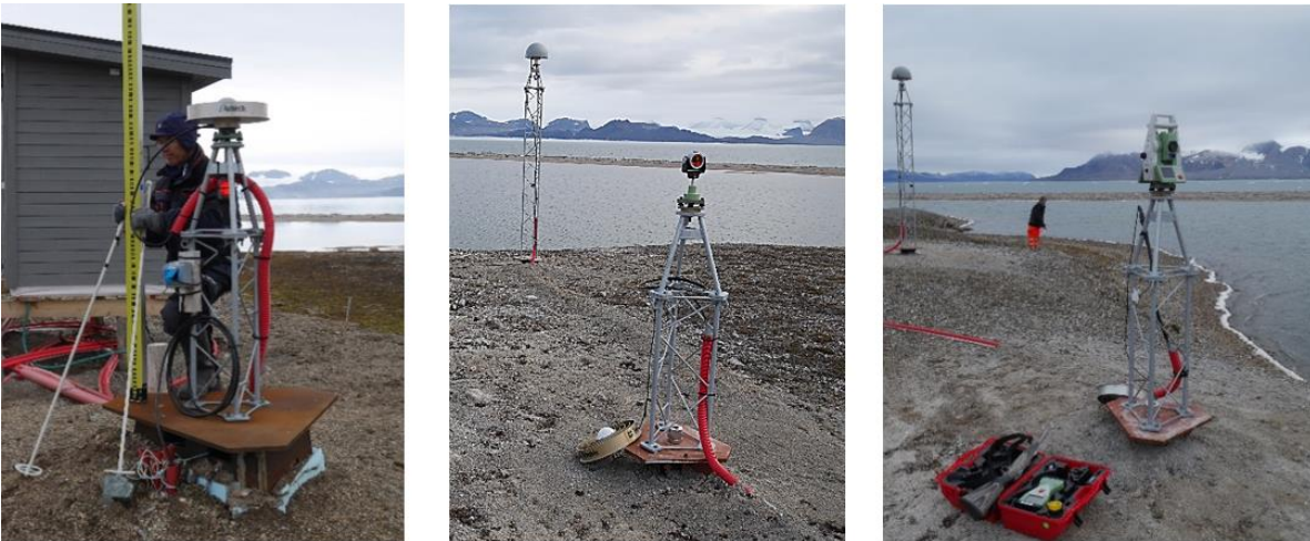
Figure 3 Control points. From left: CP2 with GNSS antenna, CP7 with prism, CP7 with total station
