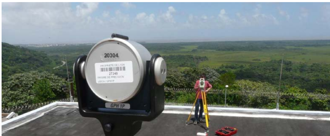
Figure 2: polygon measurements on the roof
