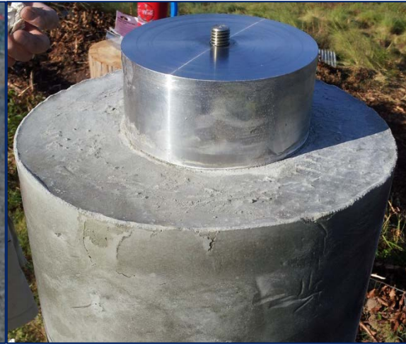
Figure 4 – CAL PIER D2 equipped with 5/8-11 stud.
