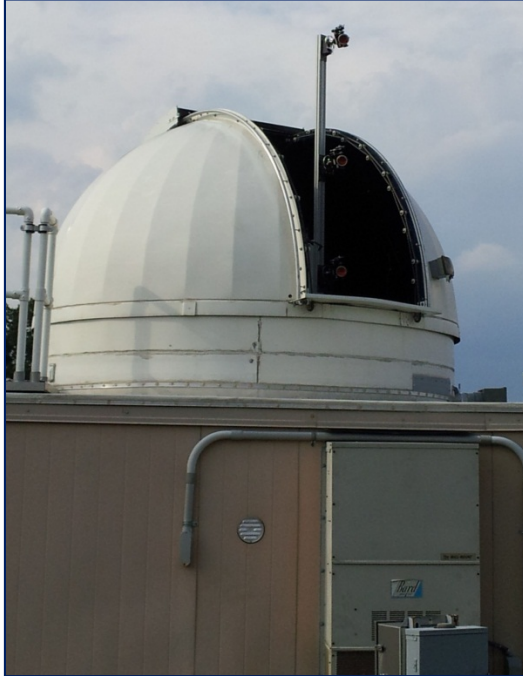
Figure 12. NGSLR w/target bar mounted vertically to the telescope. Attached targets were positioned as they scribed circles about the vertical (azimuthal) axis.
