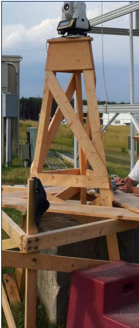
Figure 1 - Typical U.S Coast and Geodetic Survey wooden stand built over SOUTH GEOS PIER. The three-legged stand is anchored solidly into the ground and surrounded by a completely detached observer's platform.
