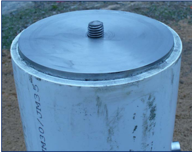
Figure 3 – NGS 1 equipped with 5/8-11 stud.
